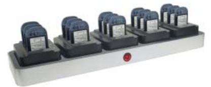
Independent “smart” charger circuit in each slot
