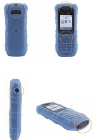
All control buttons are protected while still being accessible
